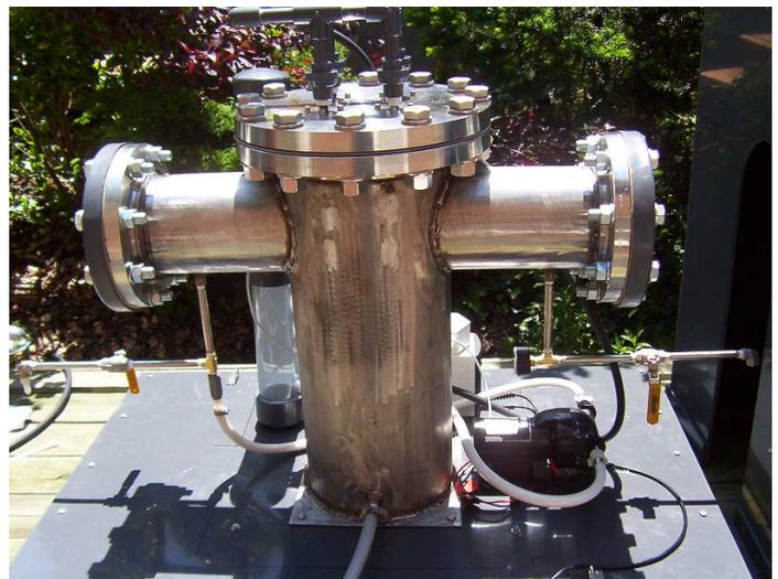
This membrane degassifier can remove 99.5% of the inlet dissolved hydrogen sulfide for a water flowrate of 500 gpm. The unit is usually enclosed in a box, that has been removed for the picture.
