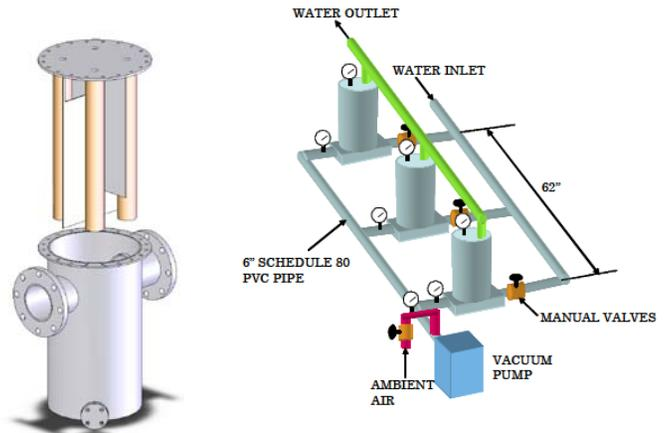
The picture below shows PRD Tech's membrane gassifier that is currently operating in Florida for removing hydrogen sulfide from water.
