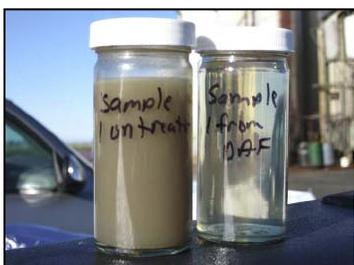
The water quality from the ADAF system is excellent. In addition, the power consumption is significantly lower than conventional DAF units. The main advantages of using PRD Tech's aeration system are:
