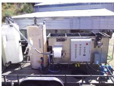
Dissolved air flotation (DAF) is a common treatment operation that has been used for a variety of industrial wastewaters for removing suspended solids (TSS), oils and greases (O&G), and biochemical oxygen demand (BOD). It is
